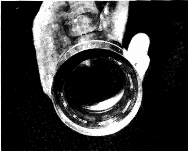
5.4. Main oil seal is integral part of screwed collar
