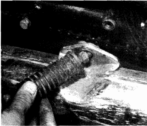
5.6a. Footrests locate with threaded lug.
