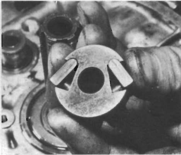
29.2. Assemble the two pawls and plungers of the gear change cam
