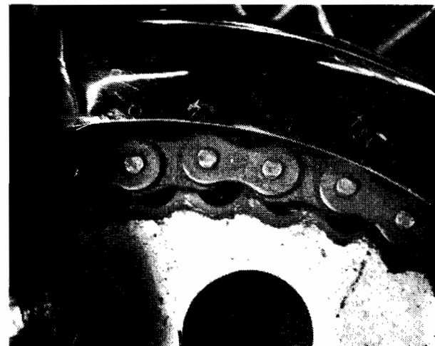
13.6. A good example of a badly worn chain
