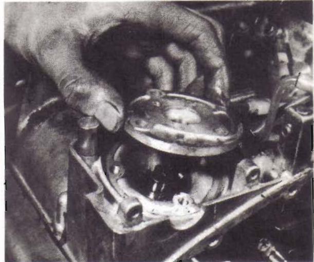
30.1a. Use a new gasket when replacing the oil pump mounting plate
