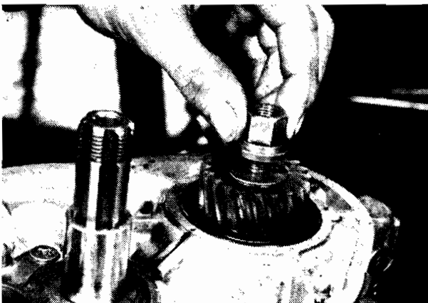
31.2b. Pinion is retained by tab washer and shouldered nut. Lock engine to tighten
