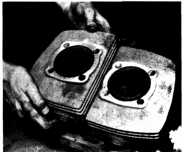
8.3. Ease cylinder barrels upwards along holding down studs
