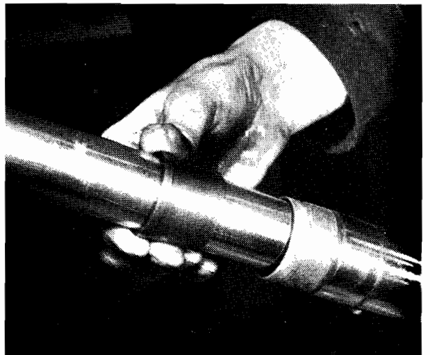
3.4. Top bush is sliding fit over inner fork tube
