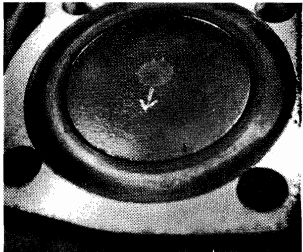
36.7. Arrow on crown must face forwards
