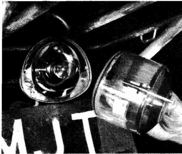
9.1. Tail and stop lamp bulb is available after removing plastic lens cover
