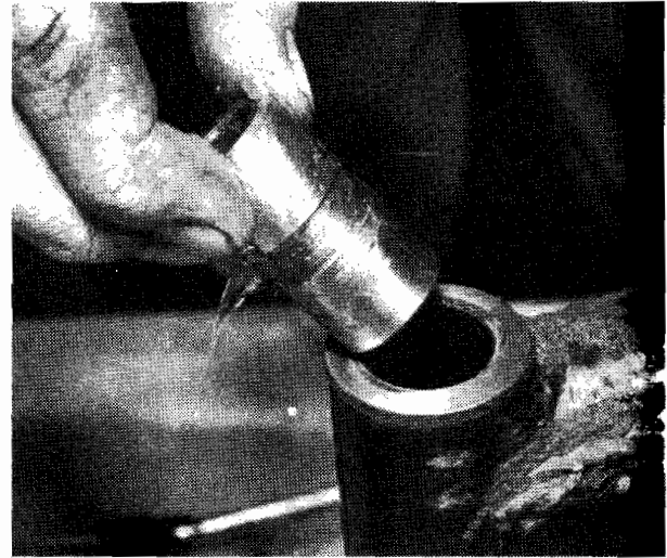
10.7. Bushes and pivot pin must be replaced to eliminate wear
