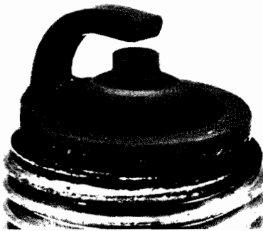
Black sooty deposits indicate an over-rich fuel/air mixture, or a malfunctioning ignition system. If no improvement is obtained, try one grade hotter plug
