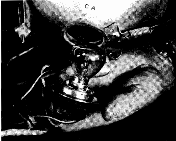
7.2. Main bulb is attached to reflector unit by rubber sleeve
