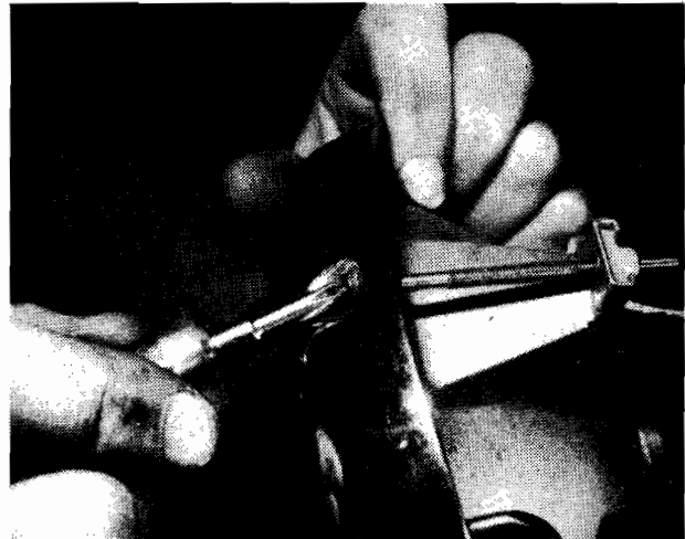
7.5. Beam alignment is effected by adjusting screw in headlamp rim
