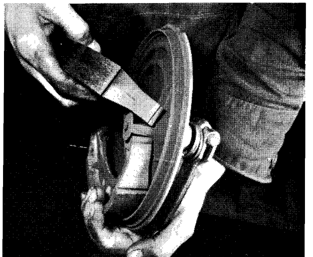
1.2. Brake shoes are separated by pulling off as shown
