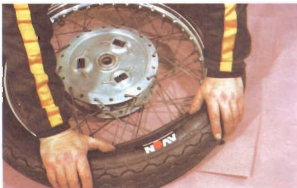
Use similar technique for second bead, finish at tyre valve position
