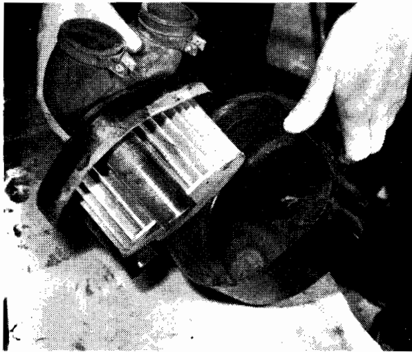
12.4 Air cleaner box contains resin-impregnated paper element
