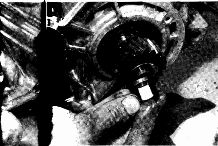
Retaining nut is shouldered and has a tab washer
