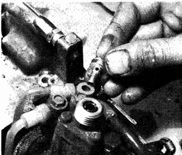
12.6a When banjo unions are disturbed, fit new sealing washers
