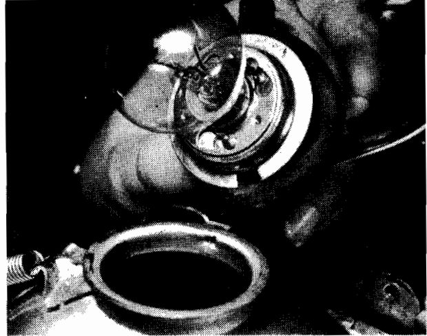
7.3. Twist bulb in holder to release. Bulb is of prefocus type
