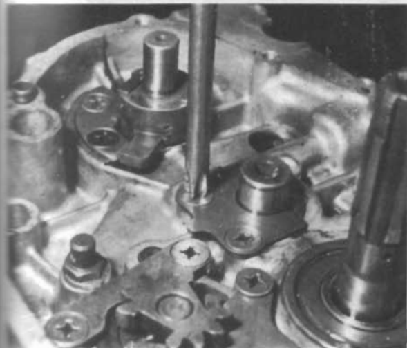
29.4. Replace the layshaft locking plate
