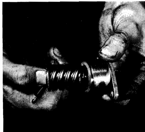
23.7. Quick start worm operates clutch. Grease well
