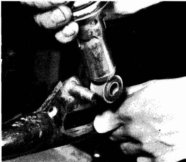
10.4. Rear suspension units are retained on studs by dome nuts
